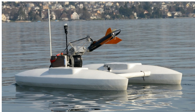
Fig. 1: Lizbeth, our limnological ASV, during a sampling mission on Lake Zurich. The probe is in its parking position out of the water.
